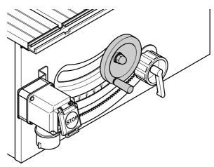
To compensate for possible play in the blade height setting mechanism, always raise the blade to the desired position.
